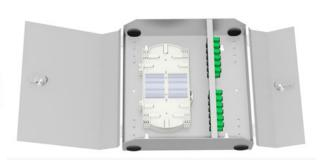
The Optical Termination Box (OTB) consists of three sections: the Pigtail and Cable Inlet, the Splice Tray, and the Patch Cord compartment. The Splice Tray is located in one section of the box, while the Patch Cord is situated in another. The layout of the incoming cables should allow easy access for installation, maintenance, and the addition of extra secondary cables.
